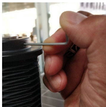
Loosen the tiny hex-bolt that keep the spindle cover in place.
