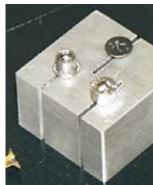
Fig. 3: Special holder for cutting screws
