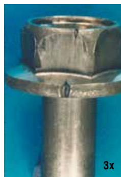
Fig. 7a: Split in head of carbon steel bolt caused by a seam.
