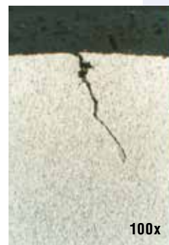
Fig. 7b: Traverse section of the seam in the fig. 7a. Echant: 3% Nital
