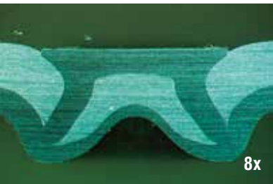
Riveted joint, steel rivet in aluminium
