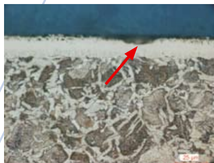
Fig. 2: Without edge retention, the layer is not in focus at high magnification
