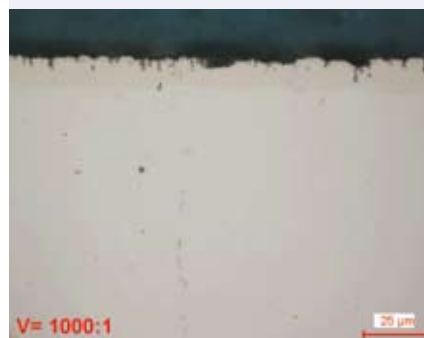
Fig.14: Alloy steel (16MnCr5N) salt bath nitrocarburised, mounted without copper foil. There is flaking of the nitride layer and the thin oxide layer can not be distinguished from mounting resin.
